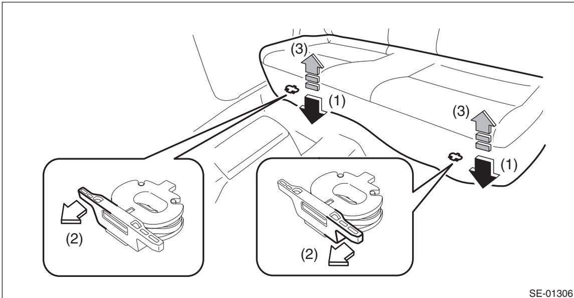
(4) Remove the hook (A) by pushing it back while lifting the front side of the rear seat cushion, and remove the rear seat cushion.
